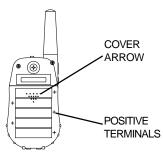
Insert five AAA batteries (positive (+) end toward right side begining at top and alternating positive terminals as shown). The following guidelines will improve performance and provide longer operating times for the GMRS9010-2:
